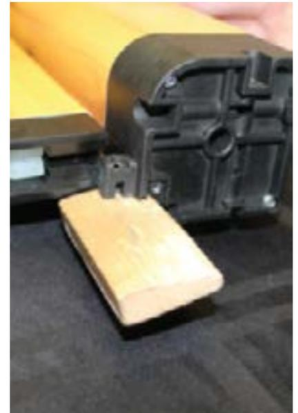
\* Use a wedge to open the slot in the housing wide enough to allow the zipper to be removed
