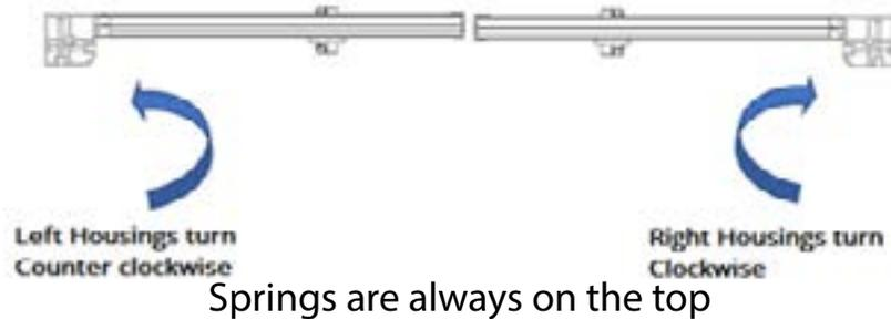
LEFT pull bar close to body, spring on right
