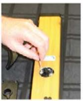
Remove the lower endcap, the back of the handle and remove brake rod assembly from the bottom
