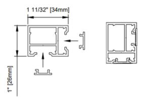
Top track can be turned 180° end to end as required for installation
