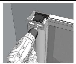
Do not rotate at full speed of drill as this will cause gears to overheat. Use low gear on drill. Caution: Do not over tension! Never apply more than 100 turns to the Spring. 20:1 gear ratio (20 turns on gearbox = 1 on spring)
