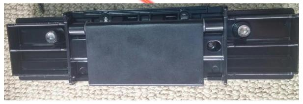
Unscrew and remove the endcaps from the pull bar – 4 screws on each end
