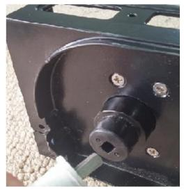
\*Match mesh spline to the roll tube
