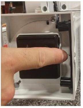
Slide the pull bar onto the mesh spline then tighten the spring
